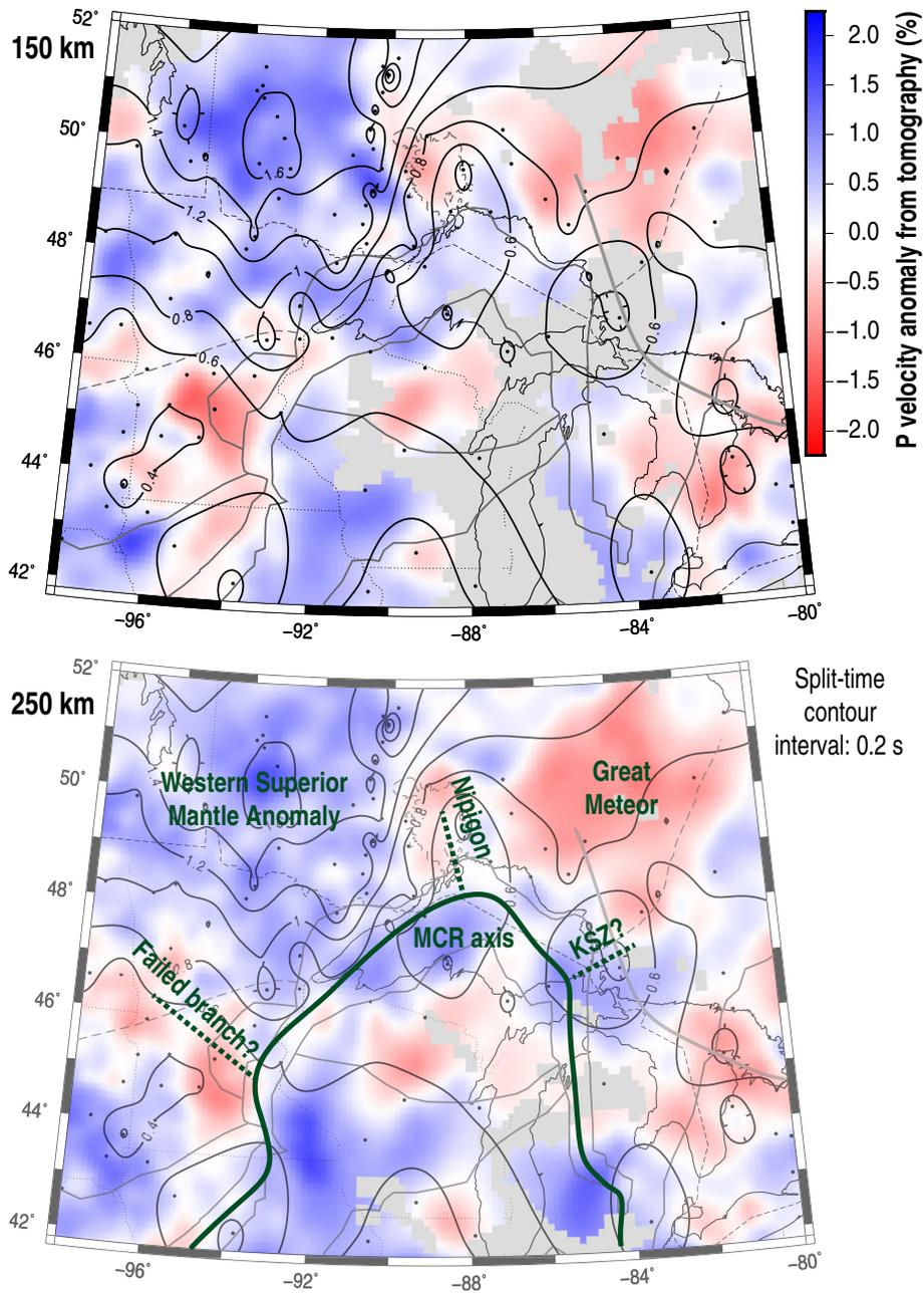
**Fig. 13.** Contours of split time in seconds (black) overlain on tomographic P velocities at 150 km depth (top) and 250 km depth (bottom) from the teleseismic model of Frederiksen et al. (2013a); black dots are locations of stations used to obtain the contours. Light grey regions indicate that the tomographic model lacks ray coverage. Dark grey lines are tectonic boundaries (see Fig. 1). The 250 km slice is overlain with interpretation (see text for details).
