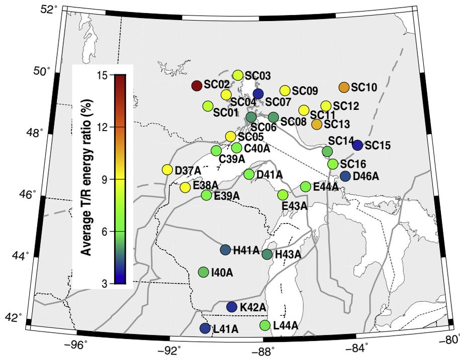
Fig. 4. Average ratio of transverse to radial energy at each station, for all events of quality  $\geq 3$ . This ratio is a direct measure of the effect of anisotropy on the SKS and SKKS traces.
