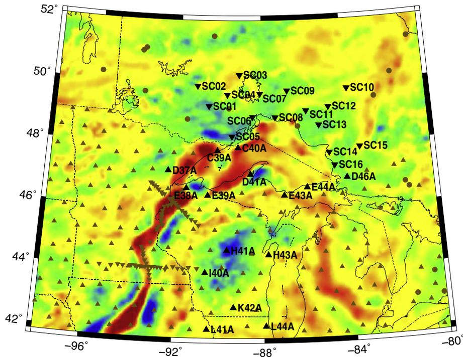
**Fig. 2.** Seismic instrumentation in the study area, overlain on Bouguer gravity (Tanner and Members of the Committee for the Gravity Anomaly Map of North America, 1988). Black symbols show sites used in this study. Inverted triangles: Superior Province Rifting Earthscope Experiment (SPREE) instruments; upright triangles: Earthscope Transportable Array instruments; circles: Canadian National Seismograph Network instruments.
