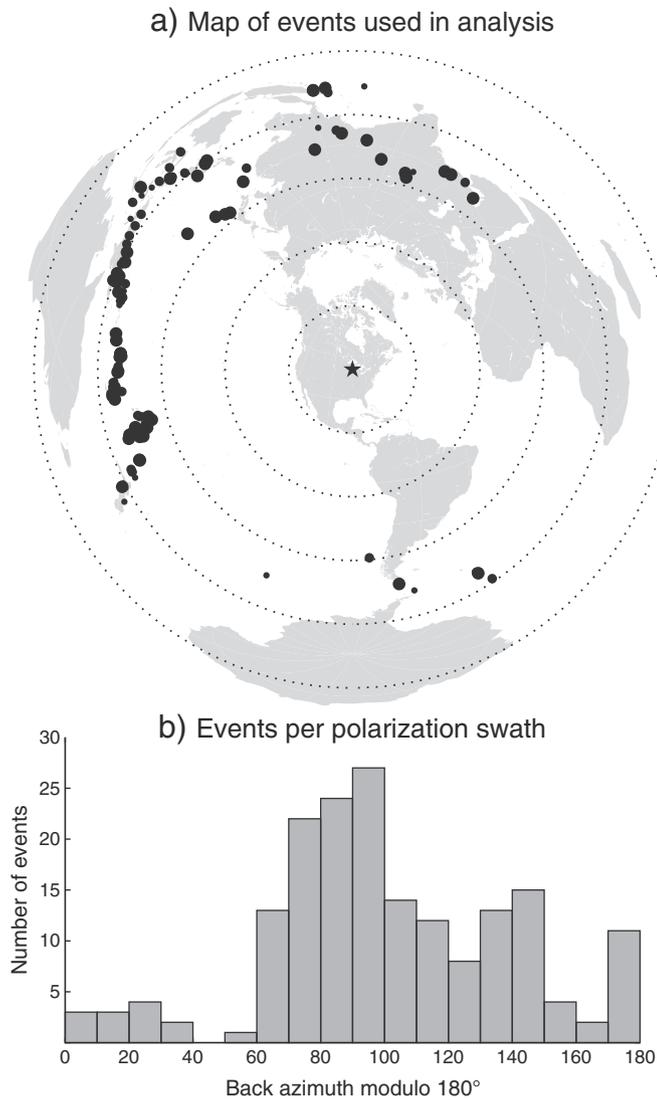
**Fig. 3.** a) Locations of events used in the shear-wave splitting analysis and judged to be of quality 3 (out of 5) or greater. Larger circles represent higher-quality events; the star indicates the approximate centre of the study area. b) Histogram of the events in (a), binned by the associated polarization direction.
