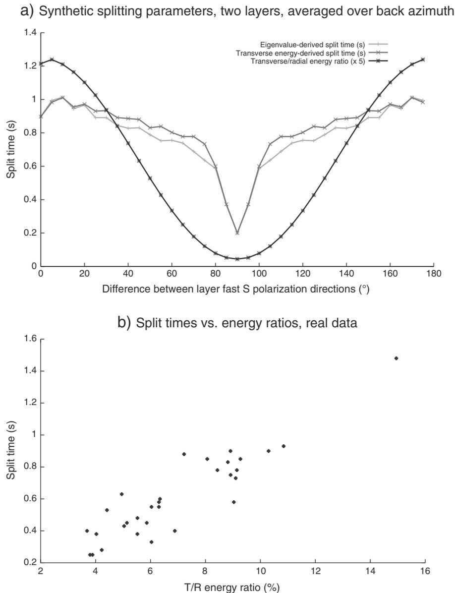
**Fig. 14.** a) Synthetic directionally-averaged split times and transverse/radial (T/R) energy ratios for a two-layer model in which the upper layer has a split time of 0.4 s and the lower layer has a split time of 0.6 s, for a range of angles between the two layers' fast polarization directions. b) Split times plotted against T/R ratios for real data.
