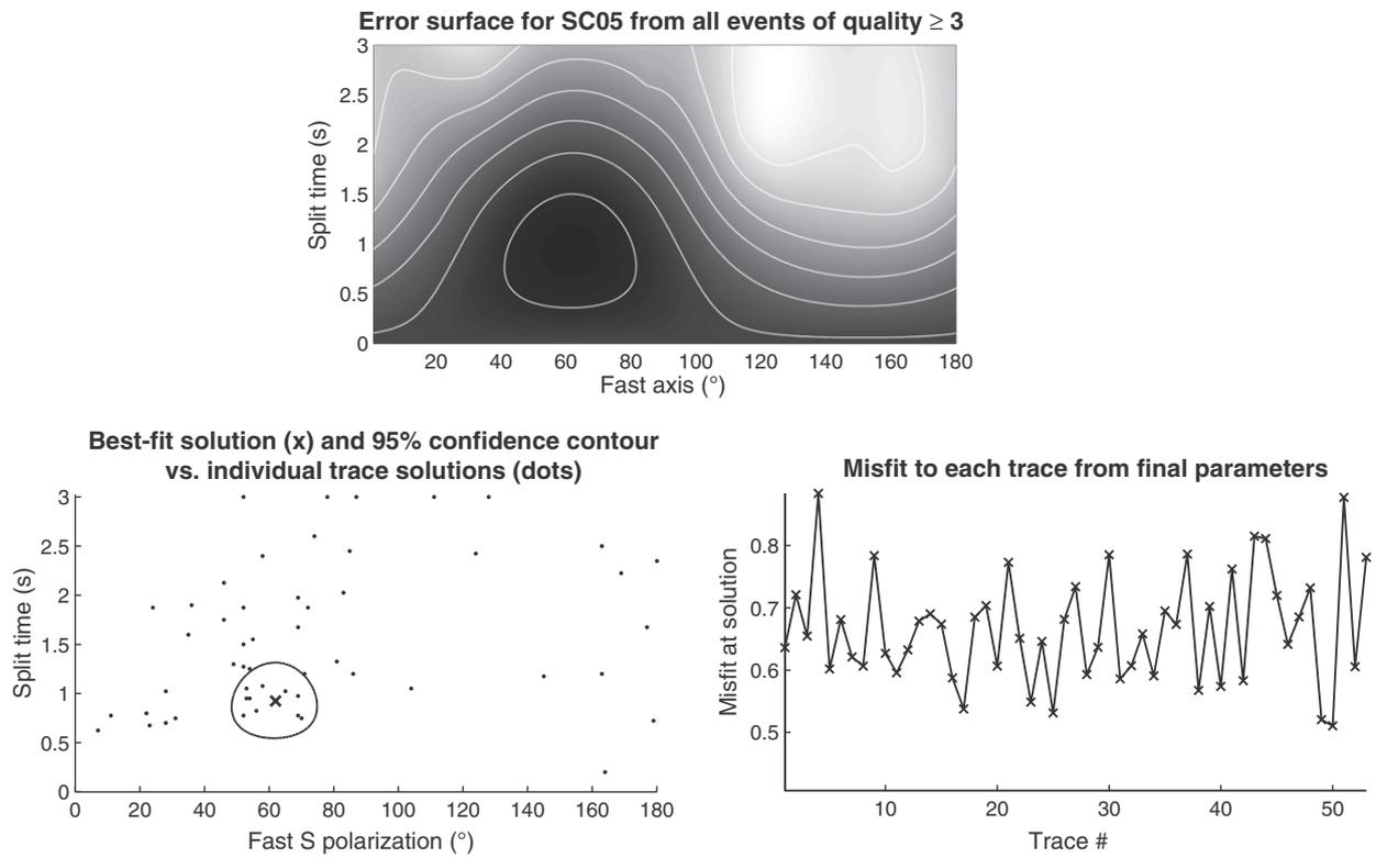
**Fig. 8.** Top: final misfit-surface stack for events of quality  $\geq 3$  at station SC05, formed by stacking all of the swath stacks in Fig. 7 with equal weight. Bottom left: best-fit solution and 95% error contour, compared to the individual-event solutions (dots). Bottom right: scaled misfit of each individual trace to the best-fit solution.
