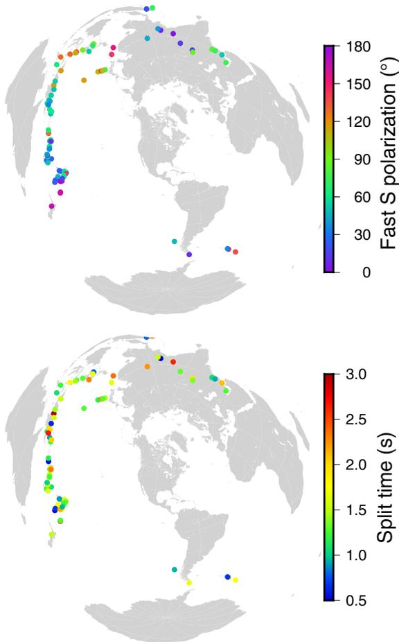
**Fig. 12.** Fast polarization directions (top panel) and split times (bottom panel) for individual events, averaged over all stations. The fast polarization directions show coherent spatial variations indicating a deep-mantle influence.
