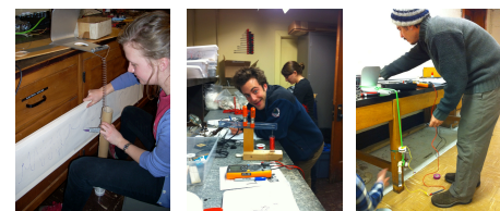
Under- and graduate students build their own seismometer in three steps: 1) mechanical, 2) mechanical → electrical, 3) analogue → digital.
